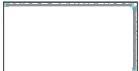
Panels are now ready for shower cubicle to be fitted if required. Please fix through panel into wall behind for secure fixing.
