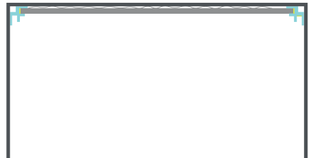
Push panel into internal corner and press against wall firmly, clean any excess silicone from corner.
