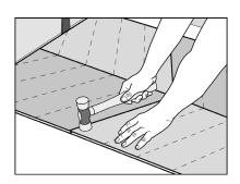
**5.** Create the required expansion by placing 3/8" (10mm) spacers between the flooring assembly and the walls. Do not remove the spacers until the installation is complete
