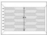
**2.** Identify the direction the chevron planks are to be installed lengthwise. Divide the width of the room by the width of one plank (302 mm). This gives you the number of rows of planks. If one row is less than a full plank (302 mm), you may need to trim the first and last row to balance out the room.
